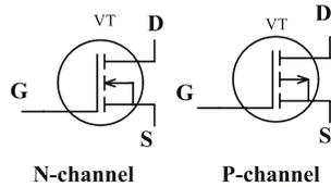
**Figure 5.45.** Field-effect transistor schematic symbol
