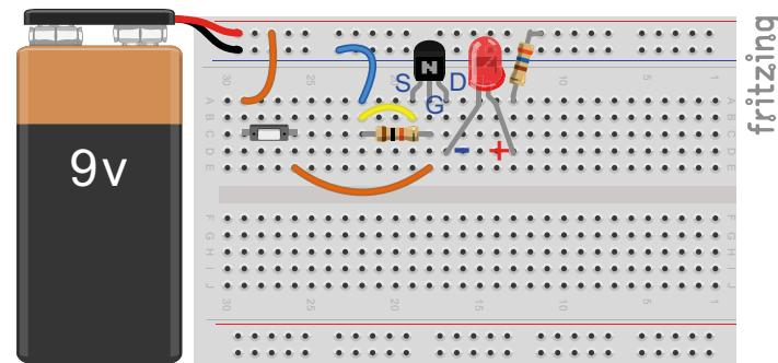
**Figure 5.47.** Field-effect transistor – electronic switch
