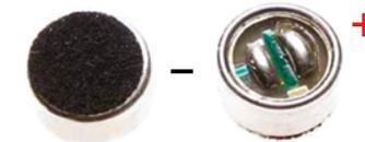
Figure 5.51. Electret microphone
