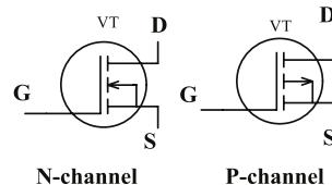
**Figure 5.45.** Field-effect transistor schematic symbol
