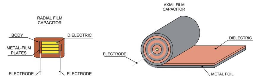
**Figure 3.12.** Construction of axial and radial film capacitors
