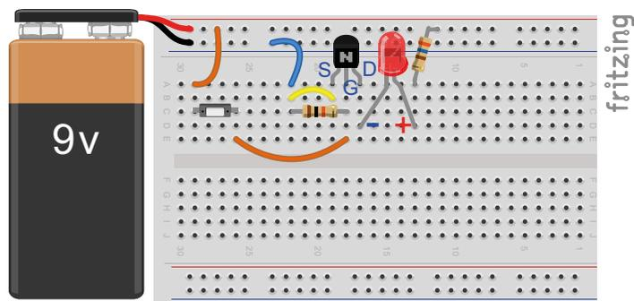
Figure 5.47. Field-effect transistor – electronic switch
