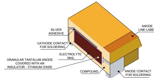
Figure 3.10. Structure of tantalum capacitor
