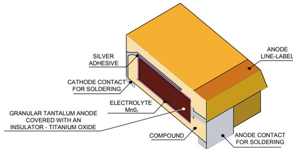
**Figure 3.10.** Structure of tantalum capacitor
