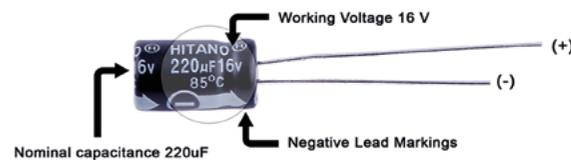
**Figure 3.11.** Markings on an electrolytic capacitor
