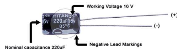
Figure 3.11. Markings on an electrolytic capacitor
