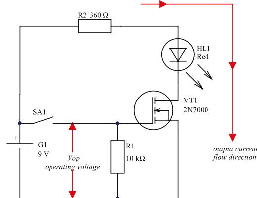
**Figure 5.46.** An FET as an electronic switch
