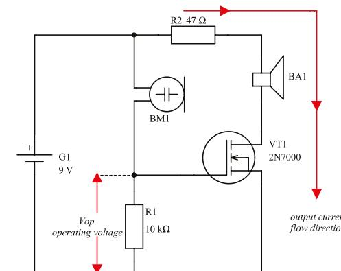
Figure 5.50. Connecting an electret microphone to a transistor
