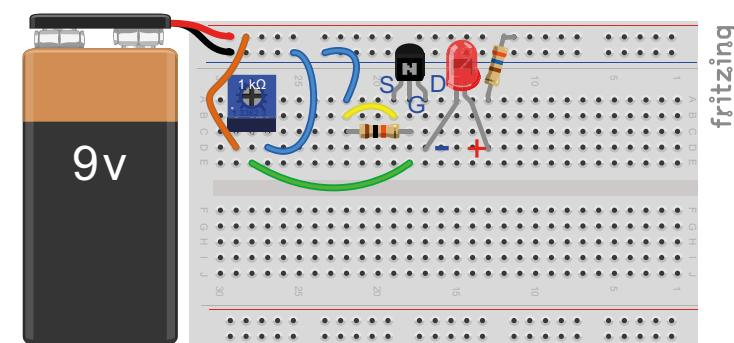
**Figure 5.49.** Adjusting the gate voltage
