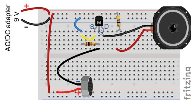
**Figure 5.52.** Connecting a microphone to FET
