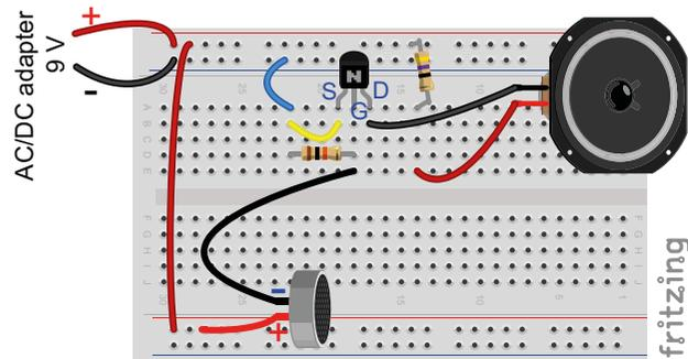
Figure 5.52. Connecting a microphone to FET
